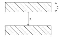
Diffusion is drawn in green, and can be referred to in Magic as either **diffusion** or **green**. It has a minimum width of 2 units and a minimum spacing of 3 units.
