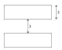
There is only one layer of metal, and it is drawn in blue. Magic accepts the names **metal** or **blue** for this layer. Metal must always be at least 3 units wide and must be
