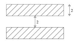
Polysilicon is drawn in red, and can be referred to in Magic as either **polysilicon** or **red**. It has a minimum width of 2 units and a minimum spacing of 2 units.
