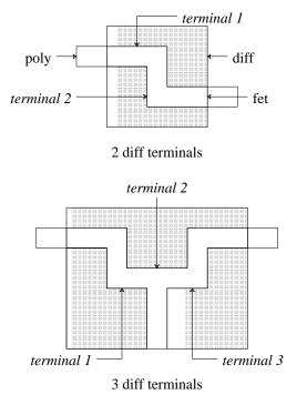
A transistor may have more than two diffusion terminals, in which case it is modeled as a collection of two-terminal transistors. If only one diffusion terminal is present, the the extractor flags this as an error and outputs a transistor with the source and drain shorted together.
