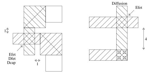
Transistors must be spaced at least 1 unit from any contact to metal, in order to keep the contact from shorting the transistor. In addition, buried contacts must be at least 4 units from enhancement transistors in the diffusion direction. This rule applies only to the side of buried contact where diffusion leaves the contact.
