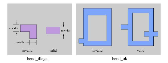
Figure 2: Examples of the maxwidth rule. The dogleg at the left would be ok in a **bend\_ok** rule, but fails in a **bend\_illegal** one, where the region's bounding box is checked. For **bend\_ok** rules, each tile in the region is checked. The left shape fails in two places: the top horizontal part is too thick and the stub at the bottom intersects the region in a shape other than a T or X.
